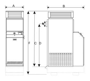
NOTE PROHEAT 30 & 60 INCLUDE A BUILT IN TANK PROHEAT 100 TANK IS OPTIONAL FITTED UNDER THE HEATER
