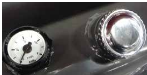
Detail tank level meter.
