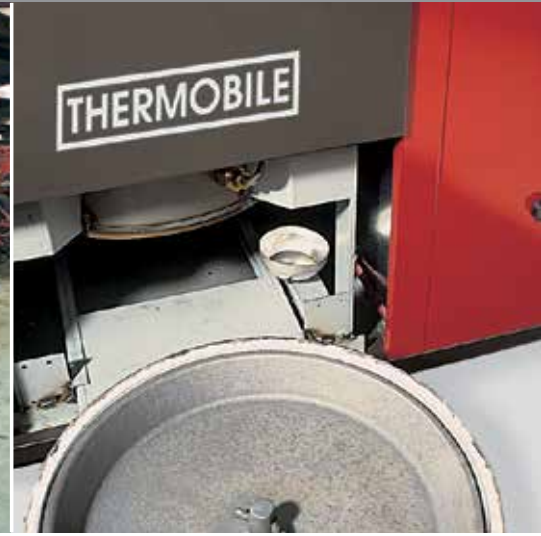
Built-in overflow protection for burner dish.
